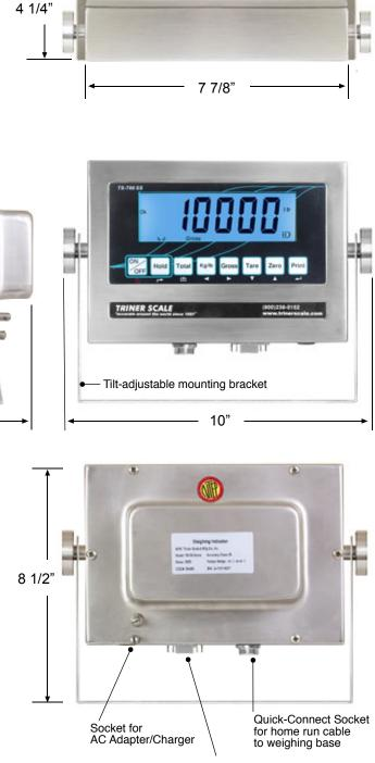
RS-232 DB-9 Socket for printer, remote display or PC
